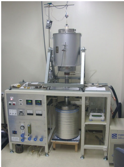
Fig. 1 Drop calorimeter combining an electric furnace and ice calorimeter.
