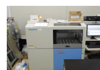
X-ray Fluorescence (Rigaku, ZSX Omnis II)
