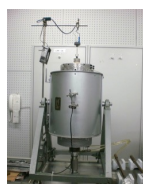
Oxygen buffer control vertical furnace (~1650°C)
