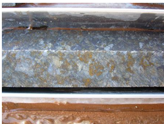
Disseminated chalcopyrite in siderite-bearing magnetite ore at Akjoujt
